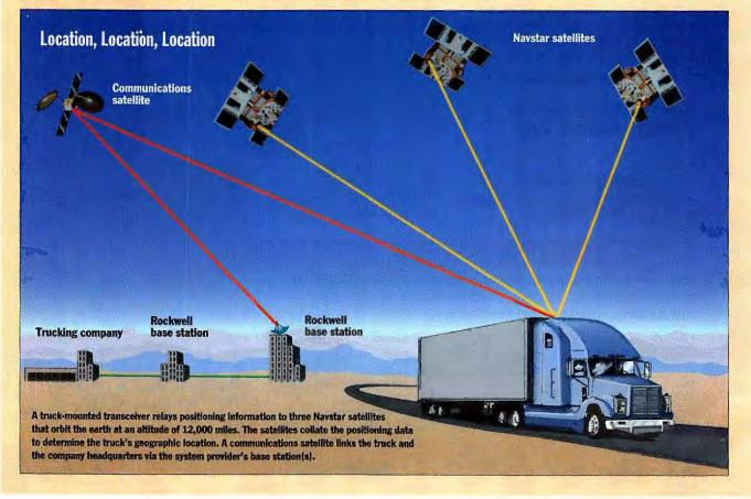
When Day & Night sends a message to a driver, the message travels through a long-distance phone carrier to Rockwell's base station. A computer located there identifies the sender and the intended receiver of the message via a data packet. Rockwell's computer then sends the message to the driver via the AMSC satellite and automatically bills the sender. Messages sent from drivers to Day & Night are routed in the same manner.
