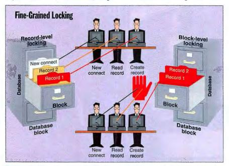
Fine-grained locking occurs on two levels within Progress, the database record, and the internal shared data structures. The figure shows how fine-grained locking services a create, a read, and a connect in parallel, while block-level locking can force the read to wait until the create is completed.
