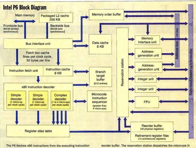
The P6 fetches x86 instructions from the executing instruction stream or from a speculative address, based on predictions by the branch target buffer. A parallel decoder converts the instructions into RISC-like micro-ops and assigns them to registers in the reorder buffer. The reservation station dispatches the micro-ops in parallel and out-of-order to five execution units. After completion, results are committed to the retirement register file and restored to original program order.
