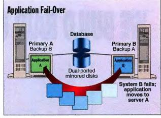
tem immediately starts the With MC/ServiceGuard, processes constantly monitor the state of each fail-over process. This pro- system. In the event of a failure, the standby system starts the scriptcess is script driven and can driven fail-over process, restarting the application on a backup system.
