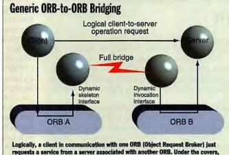
Logically, a client in communication with one over (object request prover) just requests a service from a server associated with another ORB. Under the covers, ORB A uses the new DSI (dynamic skeleton interface) to route the client's request across an inter-ORB bridge, and then ORB B issues a dynamic invocation to the server.
