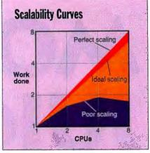
SMP coordinates multiple CPUs that share a single memory. Proportional scaling on SMP hardware is the hallmark of an enterprise-strength kernel. A poorly implemented kernel slows down when additional processors are added.
