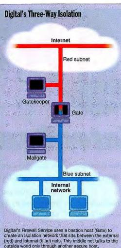
create an isolation network that sits between the external (red) and internal (blue) nets. This middle net talks to the outside world only through another secure host, Gatekeeper. It connects to the internal net either directly (for TCP/IP communications) or through a third host, Mailgate, that converts between TCP/IP and other protocols, such as DECnet.
