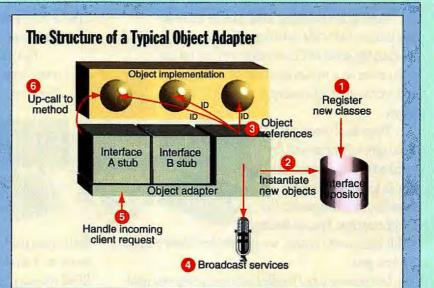
of the ORB communication stack, peels off the request, and hands it to the interface skeleton. The skeleton interprets the incoming parameters and presents them in a form that's acceptable to the object's method invocation.  Routes the up-call to the appropriate method. The object adapter is implicitly involved in the invocation of the methods described in the skeleton stubs. It may be involved in activating the implementation and can authenticate incoming requests.
