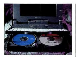
**The Panasonic V41 Multimedia Notebook** PC features an internal double-speed CD-ROM drive. The drive lies beneath the keyboard, which opens with a conveniently placed latch on the notebook's front. An adjacent slot stores a CD. The **IBM ThinkPad 755CD Notebook** and the **Aquiline Cyclone** also feature internal double-speed CD-ROM drives. However, you must remove IBM's floppy drive to
