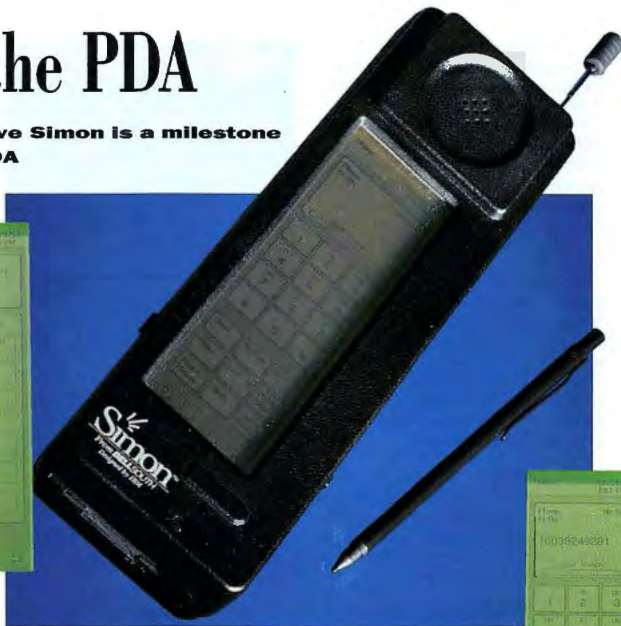
Simon looks like a large cellular phone except for its replacement of the dialing keypad with an LCD look-alike (right inset). Through the touchscreen, you operate the phone functions and a group of small PDA applications, such as the E-mail program shown (a small-screen version of Lotus cc:Mail).
