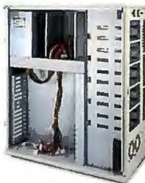
Optional all steel, US-made Monster Case features (18) 5-1/4" bays, space for 2 MBs.
