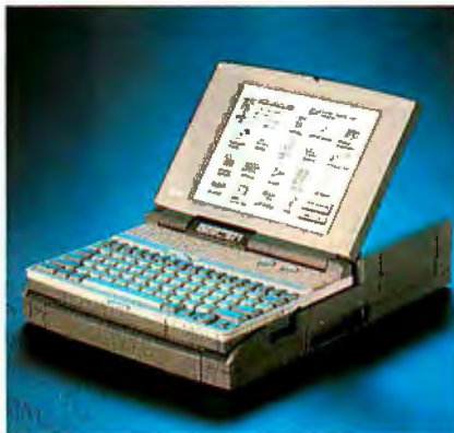
Photo 2: The docking station is almost as portable as the notebook itself. It weighs only 9 pounds with its batteries.
