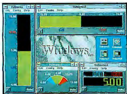
PCImeter, here displaying a digital meter (lower right corner), an analog meter (bottom center), and bar graphs (left and top).
