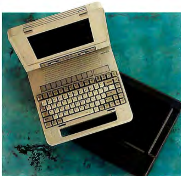
An overhead presentation system, the Mpression Notebook Presentation System combines an LCD panel with its Mport notebook computer.
