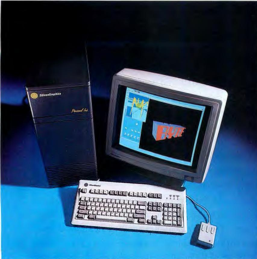
*The Silicon Graphics Personal Iris Turbo workstation. I created the BYTE logo shown on-screen as a 3-D object. The Iris can set the logo in motion, recalculating and redrawing every polygon in real time.*
