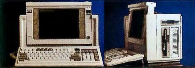
512K (286,386/sx) or 1024K (386) RAM Serial and Parallel Ports, 1.2MB or 144MB Floppy, 86-key keyboard
