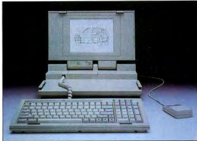
*The Altima Two is a 16-MHz 286 laptop with VGA resolution and a removable full-size 101-key keyboard.*
