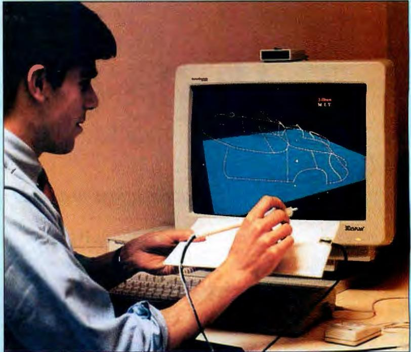
*Using 3-Draw to design an automobile body. One of its creators, Andrew Roberts, is holding the object sensor—the palette—in one hand and the drawing stylus in the other.*
