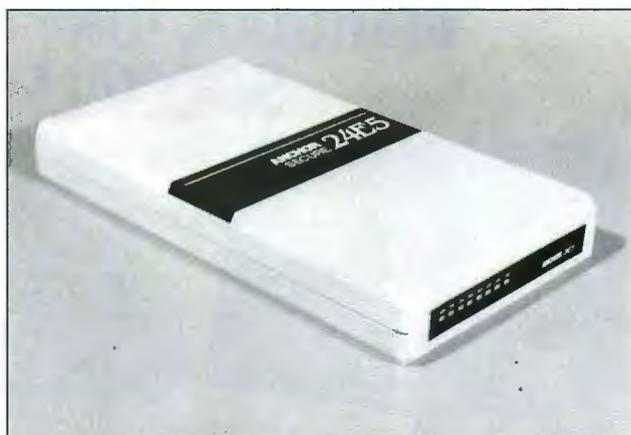
*You can program Anchor's 24E5 Secure modem to support passwords and other security features for up to 64 users. Operating in MNP-level-5 mode with data compression, throughput speed can approach 4800 bps.*
