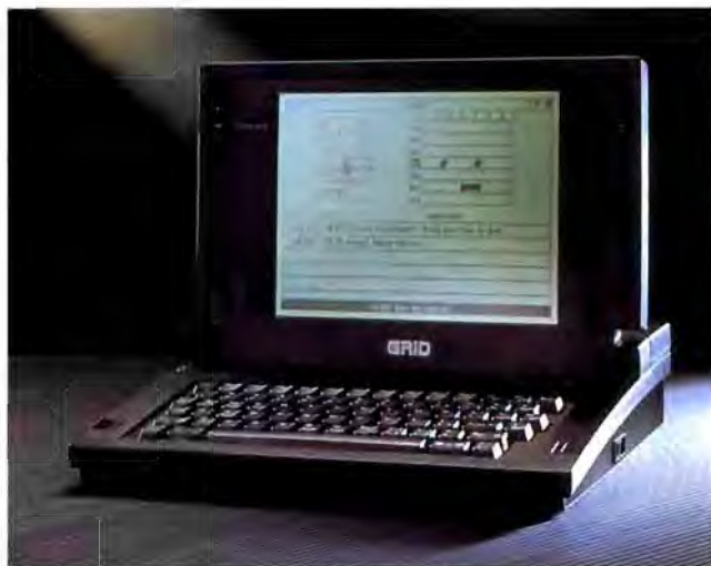
The GRiDLite XL, with a 20-megabyte drive, weighs 9½ pounds.
