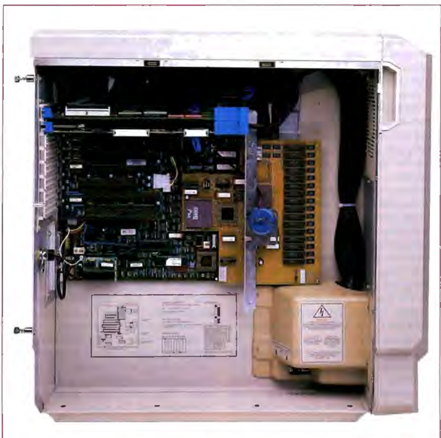
Photo 2: With only SCSI and run-length-limited disk drive controllers in two of the eight MCA slots, the inside of the VX FT Server looks empty. Note the large daughtercard on which the 80486 CPU sits. Apricot plans to integrate the CPU on the motherboard sometime in the future.
