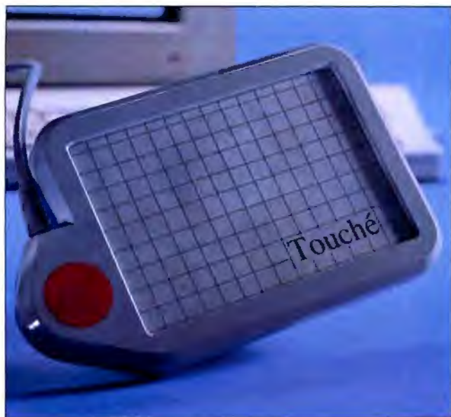
Touché, a touch tablet with a clear glass surface, provides absolute cursor control and mouse emulation.
