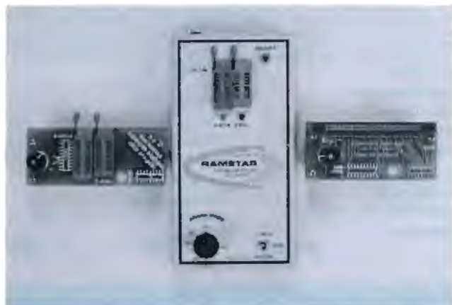
The SIMM/SIP and 4-By adapters plug into the 1-megabit test socket of the Fast RAMstar.
