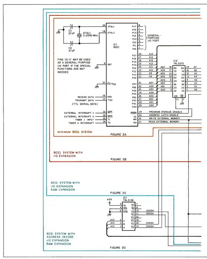
Figure 2: Growing an 8031 system. (a) A minimum configuration, (b) minimum system with I/O expansion, (c) system with I/O and RAM expansion, and (d) system with address decode logic and even more RAM and I/O.
