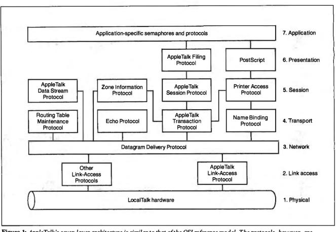
Figure 1: AppleTalk's seven-layer architecture is similar to that of the OSI reference model. The protocols, however, are proprietary.
