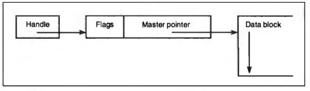
**Figure 3a:** A relocatable memory block under the Macintosh operating system. Flag bits are stored in the high bits of the master pointer. This saves space, but it doesn't work in a 32-bit environment.
