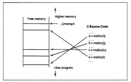
**Figure 1:** The 8088 version of BYTE Small-C handles memory allocation as an upward-growing stack tracked by the global variable \_Umemptr. Memory blocks (left) allocated by the source code (right) must be freed (using the free() function) in the reverse order to how they were allocated (i.e., the block that d points to must be released before the block that c points to). BYTE's Small-C for the Mac removes this restriction.
