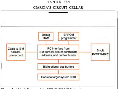
Figure 3: A block diagram of the DDT-51 8031/8051 development system.
