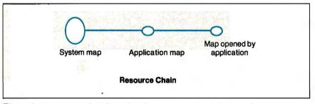
**Figure 2a:** The original MultiFinder plan for sharing resources involves searching a resource chain like this one.
