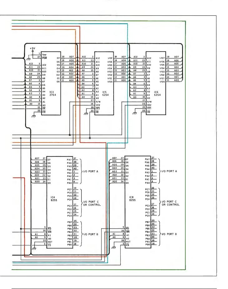
gram memory addressed by the program counter (PC), 64K bytes of external data memory addressed by the data pointer (DPTR), and the on-chip internal data memory addressed in several different ways. Each instruction implies a particular address space, so you have to know where your data resides to select the right instruction.
