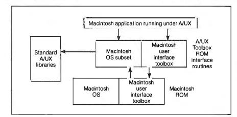
curs when the CPU executes an instruction that begins with the hexadecimal digit A. The CPU then transfers through an exception vector to a routine that handles the A-line trap. A/UX also uses the A-line trap mechanism to access the Mac ROM.
