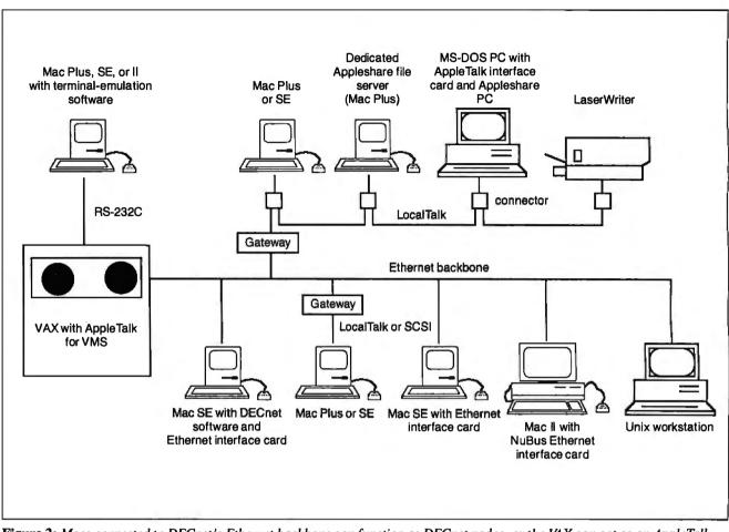
**Figure 2:** Macs connected to DECnet's Ethernet backbone can function as DECnet nodes, or the VAX can act as an AppleTalk file server.
