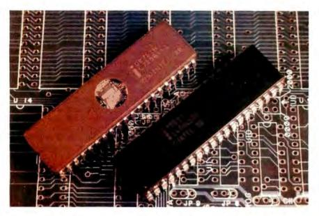
Microcontrollers are used in keyboard and disk interfaces and in numerous other devices. Here's a tutorial on the 8031/8051 microcontroller family.
