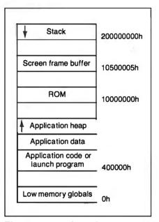
Figure 2: Except for the low-memory globals, none of the addresses that A/UX uses are the same as the ones used by the native Mac operating system. This doesn't matter, since everything is referenced through pointers in memory.
