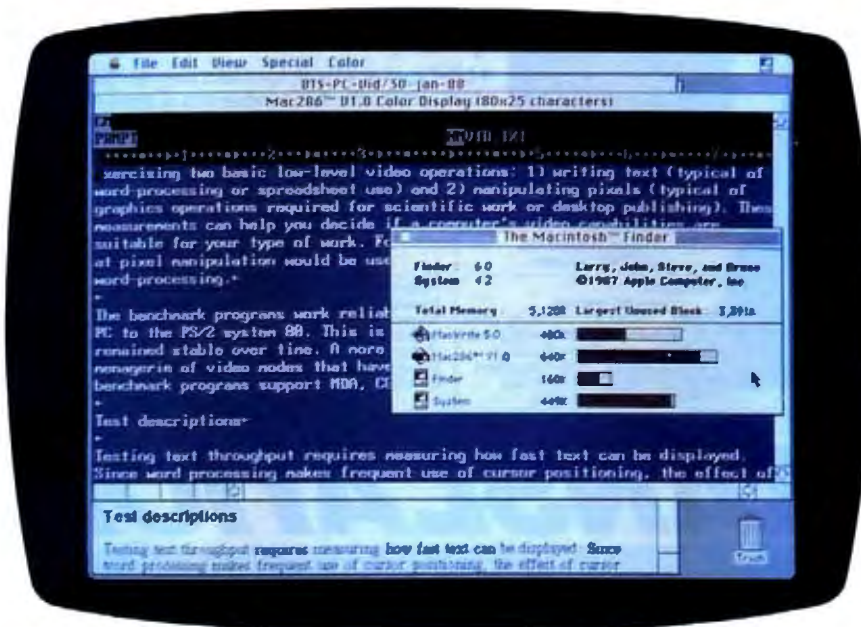
Photo 1: The Mac286 runs under MultiFinder on a Mac II with a 256-color display. The MacWrite document shown was just converted to a text-only file called VID.TXT and was copied to Mac286's drive C using the DOS command COPY D:VID.TXT C:. The document was then opened as it would be with XyWrite.
