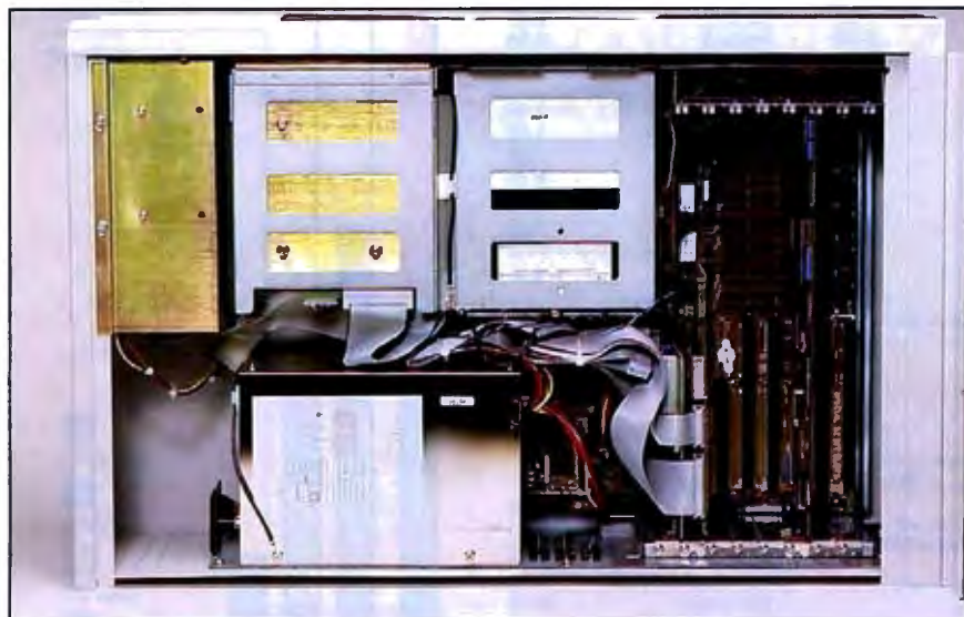
Photo 1: The internal view of the 20386 clearly shows the case-within-a-case construction that allows extra space for additional disk drives.
