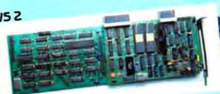
This System is equipped with the SandStar™ Floppy Drive Controller Card. The Card can control, in addition to the Hard Disc Drive, two floppy drives mounted inside your PC and optionally two additional 5¼" or 8" drives mounted externally. This leaves three system slots for other expansion boards.
