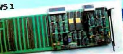
This System is equipped with the SandStar™ Multi-tion card. In addition to the Hard Disc Controller module, you can add up to three other SandStar™ modules while using only one card slot. The following modules are available: Serial Port, Parallel Port, Clock Generator, Game Adaptor, and Prototyping Module.
