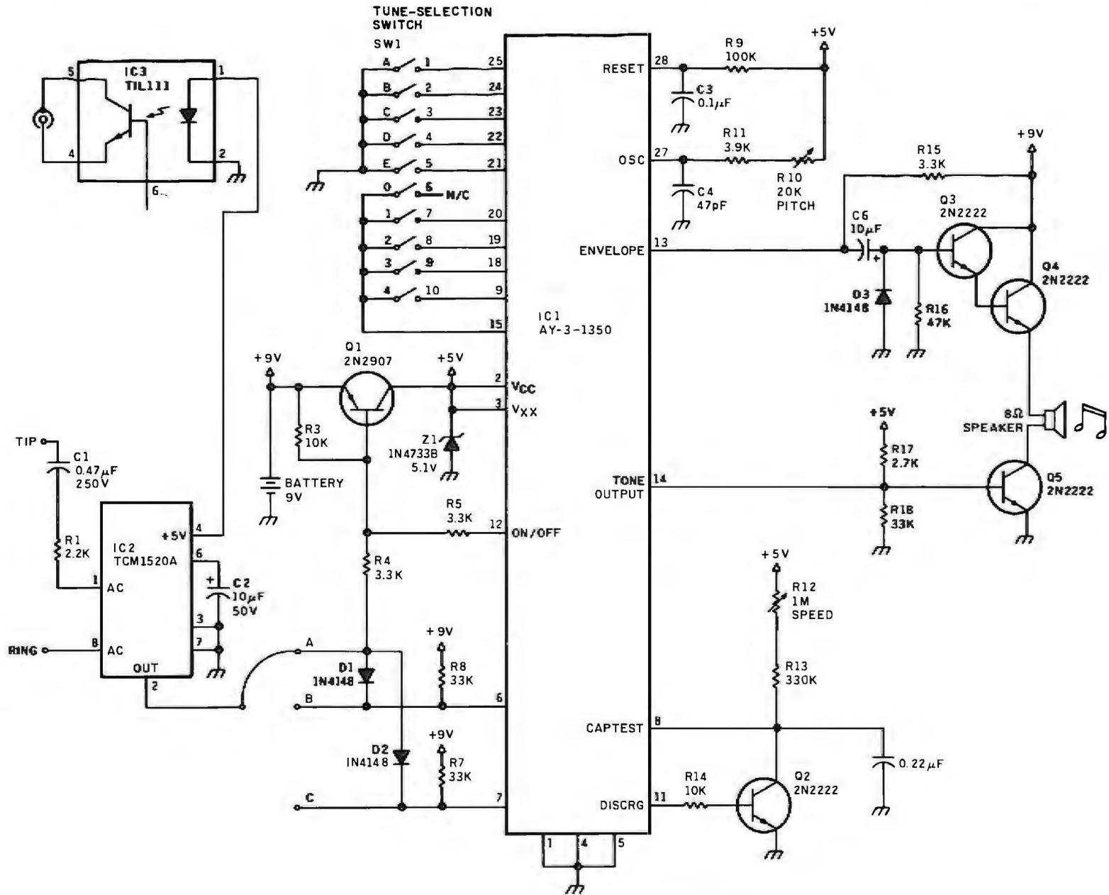
voltage between pins 1 and 8 exceeds 8.9 V (remember, the off-hook condition is a DC voltage on the line, and the series DC-blocking capacitor prevents the ring detector from seeing this voltage). While in standby mode, the impedance is approximately 1 megohm.
