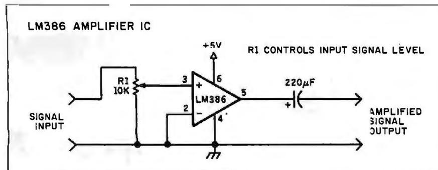
Figure 4: The sound-amplifier circuit.
