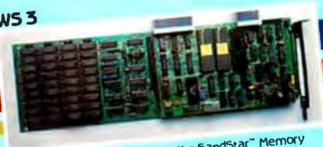
This System is equipped with the SandStar™ Memory Card. In addition to controlling the Hard Disc Drive, the Memory Card allows you to add 64K bytes to 576K bytes of memory using only one card slot.
