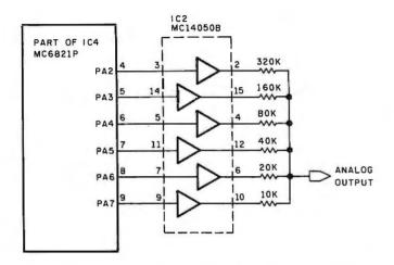
**Figure 11:** Schematic diagram of the Color Computer's digitalto-analog converter. In a rather simple scheme, the output lines of a parallel port drive a resistive adding network to provide conversion. The resulting analog signals are used for recording on a cassette, providing the video modulator with sound, and also as part of the analog-to-digital converter.
