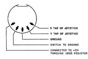
**Figure 14:** Pin designations of the Color Computer joystick connectors. The connectors will mate with a standard 5-pin DIN plug, and any signal within the A/D converter's range may be monitored under program control.
