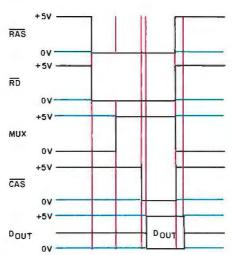
**Figure 3:**  $\overline{RAS}$ ,  $\overline{CAS}$ , and MUX timing diagram for 4116-type 16-pin dynamicmemory integrated circuit. A 14-bit address (16,384 by 1) is multiplexed <u>into</u> seven address pins. When MUX and  $\overline{RAS}$ are low, the row-address bits are read into the 4116. Later, when MUX is high and  $\overline{CAS}$  goes low, the column bits are read into the 4116, activating the data output for that memory cell.
