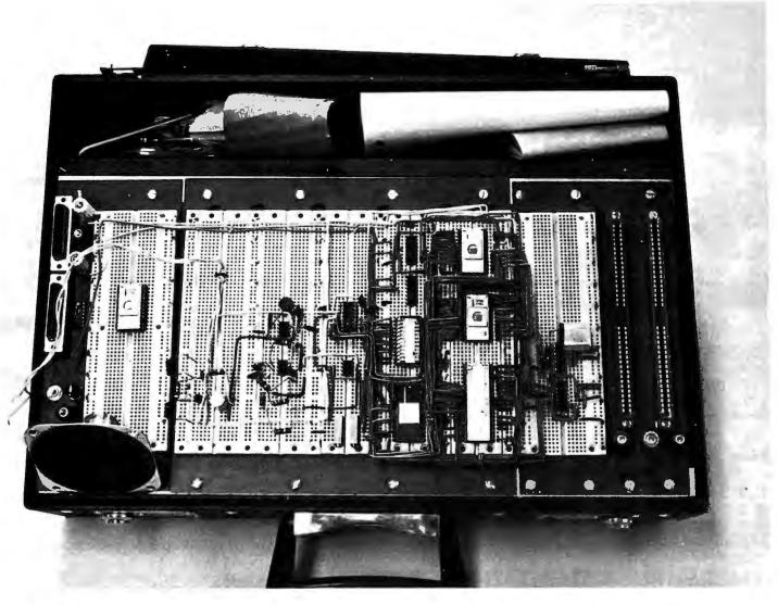
**Photo 1:** The author's microprocessor computer music system implemented in a breadboard prototype suitcase. A 2<sup>1</sup>/<sub>2</sub>-inch speaker (lower left) provides audio output for demonstrations. Best results were obtained by patching into the power amplifier of a high-fidelity receiver.
