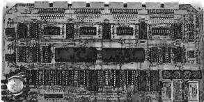
4 PORT I/O •Quad RS-232C Serial Ports, One 20mA Current Loop Port •Fully IEEE S-100 Bus Compatible •Asynchronous Communications with Z80A-Dart(TM) or
