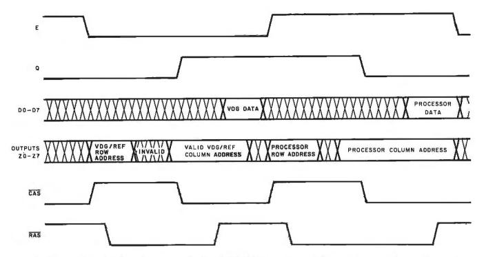
Figure 8: Diagram of a typical dynamic-memory refresh cycle. The SAM provides every dynamic memory with a signal on each row address, as required, to refresh the data contained within.
