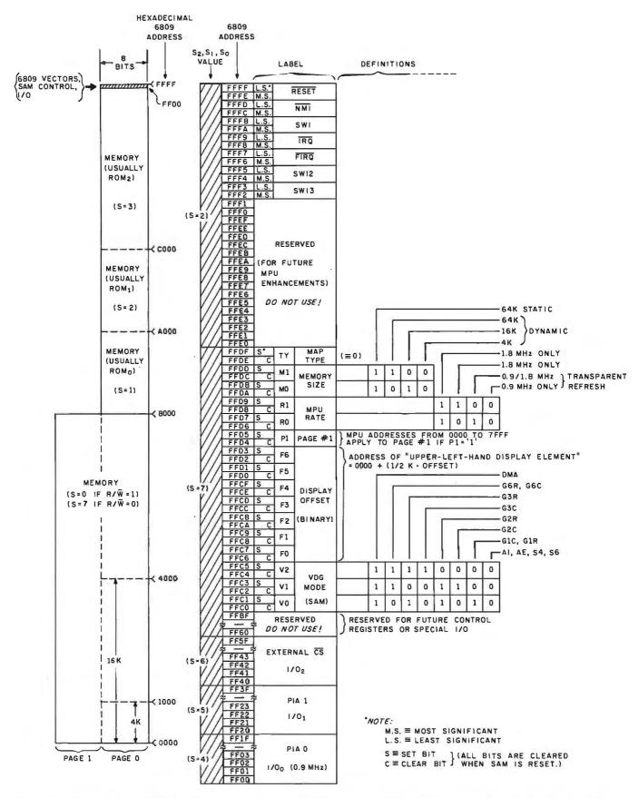
**Figure 9:** Memory map of the Color Computer address space. The general division of addresses is provided at the left, while the SAM programming registers and the processor-interrupt vectors are expanded at the right.
