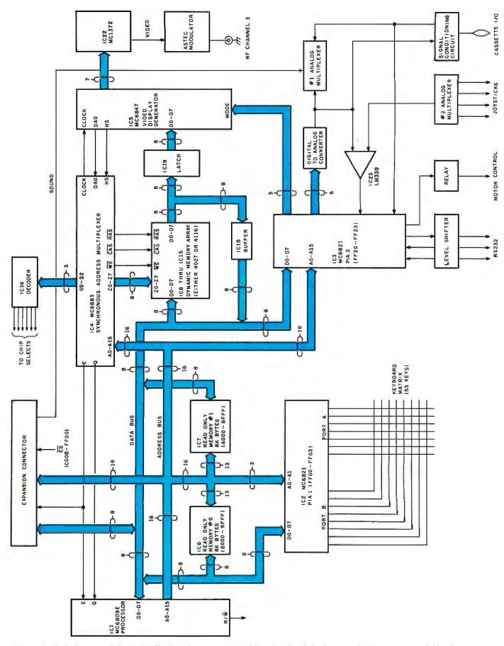
**Figure 1:** Block diagram of the Radio Shack Color Computer. Although a detailed schematic diagram is not available, the connection of the main components can be readily determined. Note that the use of large-scale integrated circuits (the microprocessor, SAM dynamic-memory handler, video-display generator, and parallel port interfaces) means that a minimum number of components is necessary to build this flexible computer.
