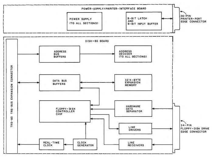
Figure 1: Block diagram of the Disk-80 expansion interface for the Radio Shack TRS-80 Model 1.
