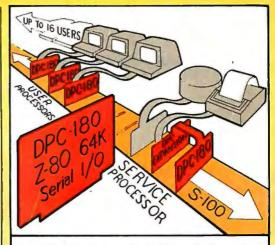
The ACE **DISCOVERY MULTIPROCESSOR** dedicates a complete, 64K Z-80 Distributed Processing single board Computer, the **dpc-180**<sup>™</sup> to each user. An expanded DPC coordinates all of the system activities.
