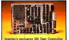
The secret behind our CompuStar DSS is its unique controller/multiplexor. It allows many terminals to "share" the resources of a single disk. So, not only can you use the DSS with your Super-Brain, you can configure multiple user stations using our new series of Compu-Star<sup>TM</sup> terminals, called Video Processing Units or VPU's<sup>TM</sup>.
