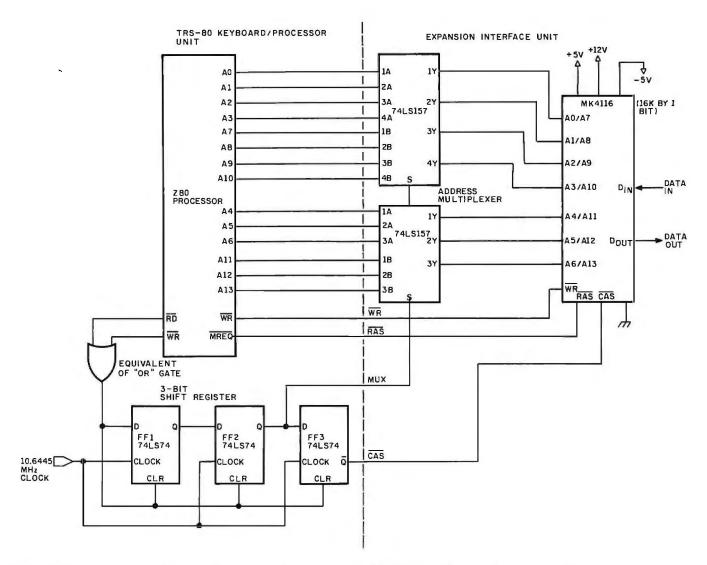
**Figure 4**: Simplified schematic diagram of the internal circuitry of the TRS-80 Model I showing the derivation of the memory-refresh logic.
