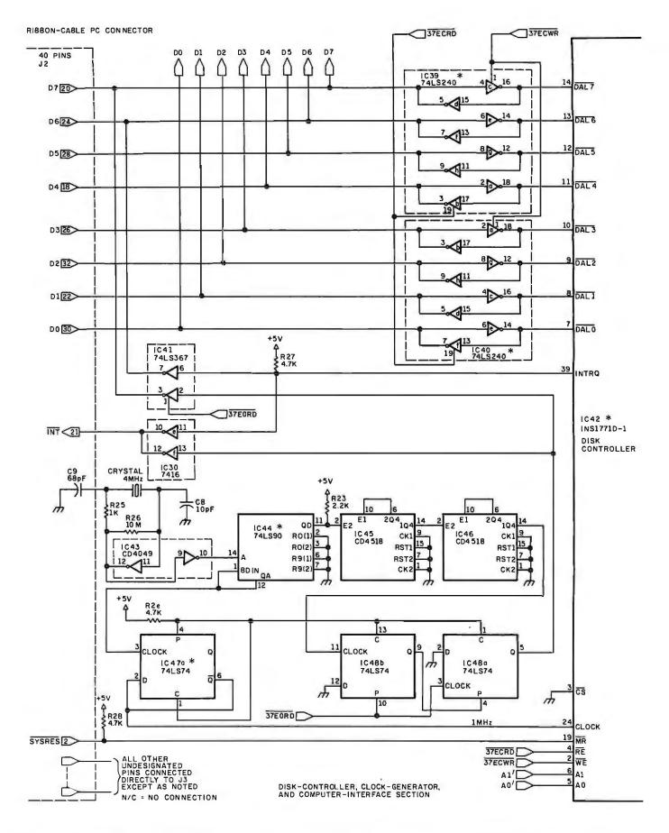
**Figure 2c:** Schematic diagram of the disk-controller, clock-generator, keyboard/processor-module-interface, external-data-separator, and disk-drive-interface sections of the Disk-80 expansion module. See figure notes on page 44.
