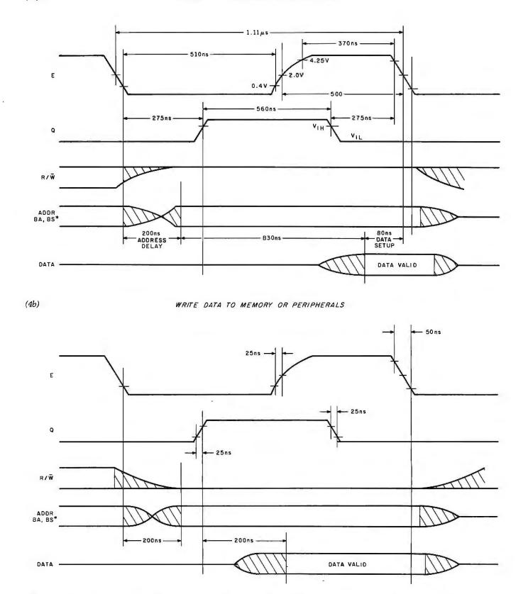
**Figure 4:** Timing diagrams for 6809 bus operations. As with the 6800, both memory and peripherals are accessed in the same way and share the same address space. The complete instruction cycle for reads (figure 4a) and writes (figure 4b) is the same: approximately  $1.1 \mu s$ .
