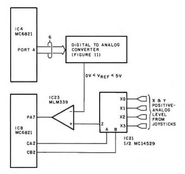
**Figure 12:** Diagram for the analog-to-digital converter circuit. Also used as the joystick interface, this circuit applies the successive-approximation method (see figure 13) to change analog signals to digital form.
