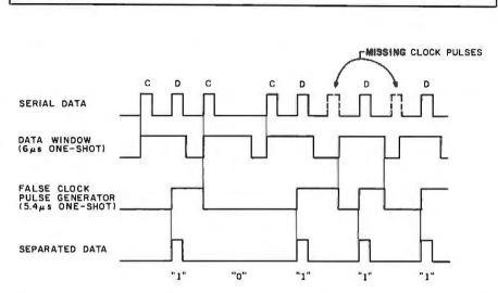
**Figure 6:** Timing diagram illustrating the operation of the external data separator shown in figure 5 on page 47. Clock pulses are denoted by the letter C, data pulses by the letter D.
