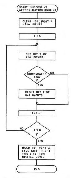
**Figure 13:** Flowchart of the successive-approximation algorithm used by the Color Computer.
