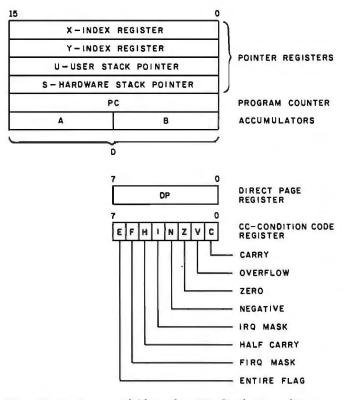
**Figure 3:** Registers available in the 6809. Similar in architecture to the 6800, the 6809 has three extra registers to facilitate memory acesses: a direct page register, a user stack register, and a second index register. The instruction set is also more robust, with the addition of 16-bit add, subtract, and multiply operations. Text continued from page 90:
