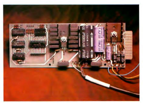
**Photo 3:** The Disk-80 power supply with the parallel printer interface. The power supply provides 1 A at +5 V, 400 mA at +12 V, and 50 mA at -5 V, and is designed for use with dynamic memories such as the 4116 that require sequenced application of power.
