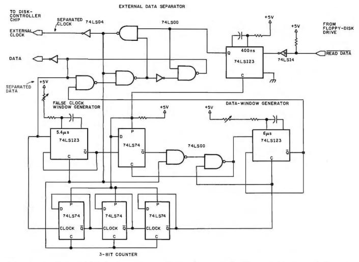
**Figure 5:** Simplified schematic diagram of a 5-inch floppy-disk external data separator. The internal data separator of the FD1771 is not recommended for use in such applications. This circuit can be added to any existing TRS-80 Expansion Interface (which does not have an external data separator) to improve performance.
