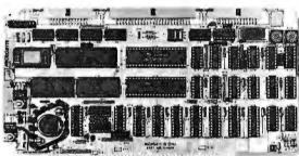
**Z-80A/I-O** •A complete single board Z-80A CPU with serial/parallel interface •Fully compatible with the proposed IEEE S-100 Bus Standard •Z-80A CPU (4MHz version of the Z-80)
