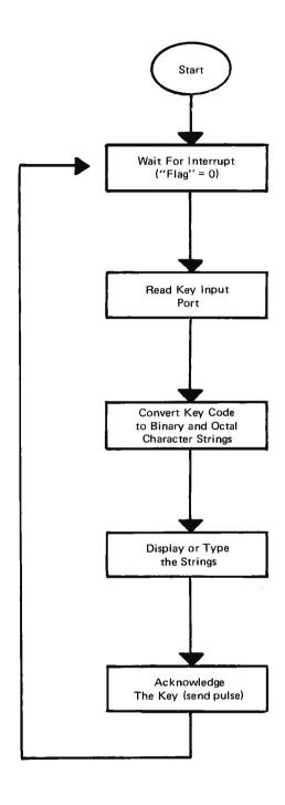
Fig. 6. Keyboard Test Program Flow Chart.
