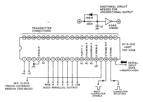
the receiver portion of the UART. Although the receiver and transmitter can be used in totally different circuits and at different baud rates, they have to operate with a common format, set by these pins.
