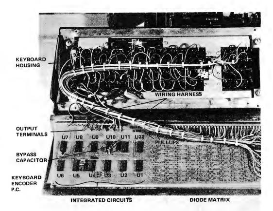
The keyboard, with bottom plate removed and encoder board out in the open. The encoder printed circuit is separated from its mounting on the bottom plate but is still attached by its wiring harness.
