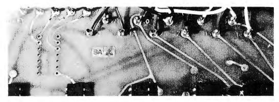
the positive supply and ground, with markings of (+) for the supply side and (-) for the ground side. In the disassembled keyboard photograph accompanying this article, the bypass capacitor is labeled. Using clip leads, the bypass capacitor often provides a handy way to apply power when first testing the board.
