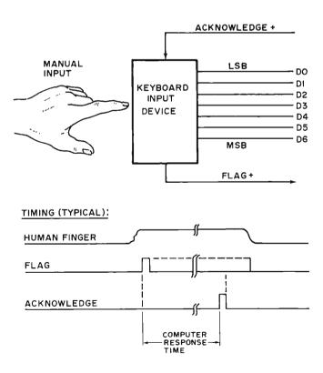
Fig. 1. Typical keyboard functions.
