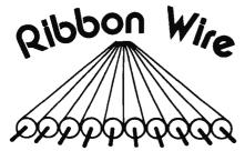
This is a flat, multiconductor wire, available in multiples of 10 conductors up to 100 conductors. Comes in 20 ft. lengths only. Cost is 1¢ per conductor foot; for example, a 20 conductor cable 20 ft. long =
