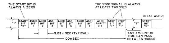
Fig. 2. 110 Baud, 100 word per minute code. "0" is a space or an open line. "1" is a mark or a shorted line.
