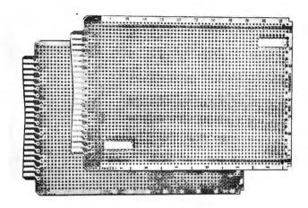
Edge connector configuration on Vector 3662A-6 Plugbord reduces insertion forces by 2-1/2 lbs.
