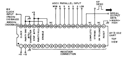
Baud circuit needs a clock of 1760 Hertz, while a 300 Baud one uses a 4800 Hertz clock and so on.
