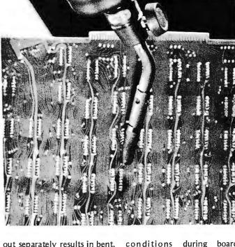
out separately results in bent, often broken leads. Devices are available which will heat all 14 or 16 pins of a small IC, but again a long time is needed to melt the solder since the total amount of energy available is limited to a small soldering pencil heating element. Most available boards are two sided and four layer boards aren't uncommon. Multi-layered boards make the required amount of energy even higher.
