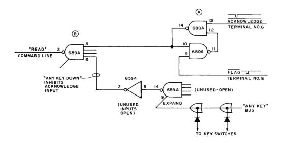
Table ΙΙ. Terminal Connections for the Sanders surplus keyboard. Terminal I.D. #5 Power (+5 volts) #6 Acknowledge (-) #7 Ground #8 Flag (-) (pulse unless REPEAT key held down) #9 Bit 0 (+) ASCII LSB #10 Bit 1 (+) #11 Bit 2 (+) #12 Bit 3 (+) #13 Bit 4 (+) #14 Bit 5 (+) #15 Bit 6 (+)
