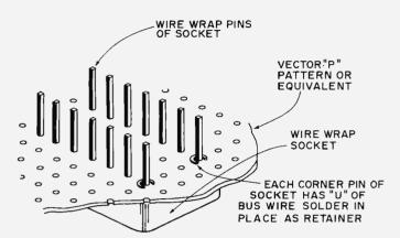
If you want to wrap up a quick project, it is often handy to use perforated board (eg: Vector "P" pattern VECTORBOARD) to mount wire wrap sockets. I have used many methods for attaching boards - rivets, bolts, epoxy glue, cyanoacrylic glue, etc. One method which I dreamed up the other day to solve the mounting problem for a small test jig may prove useful to you at some point. Simply put the socket through the perforated board, then solder each corner pin with a "U" shaped retainer made of bus
