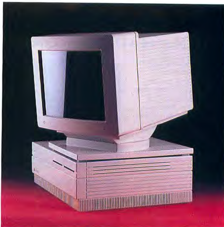
Color Performance The Mac II color monitor measures 13 inches diagonally and displays color images with a resolution of 69 dots per inch. It is shown here atop the Universal Monitor Stand.
