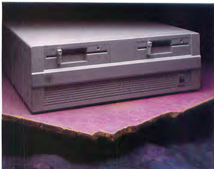
Several new hardware products provide a degree of MS-DOS compatibility. Dayna Communication's SL286, which works with the Mac SE and the Mac Plus, is an AT-class file server running MS-DOS that connects to AppleTalk.
