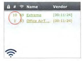
nel—usually 11. Newer phones use something called *frequency hopping technology* that allows them to leap from channel to channel, looking for the strongest one. If the phone lands on the channel you've assigned to your base station, you could get interference even after switching channels.
