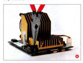
Don't assume that the processor will ship with the jumpers set correctly for your machine. The 1.467GHz Giga Designs upgrade, for example, ships with the jumpers set properly for 100MHz-bus computers. What happens when you put the card as is into a 133MHz-bus machine? The Mac won't boot.
