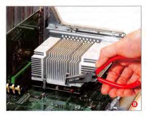
Warning: It's essential that the heat sink be evenly and firmly secured. If even one of the clips isn't properly secured, the card may overheat and damage the chip.
