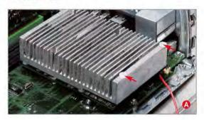
Set the fan unit on top of the spacers and secure it with the two provided screws. Make sure the fan is pointed in the proper direction—so that the air blows down on the card.
