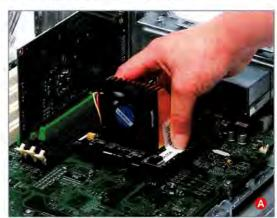
Using the screws you removed in step 2, secure the processor card. For upgrade cards such as the PowerLogix, the screws are set through the heat sink, so a magnetic screwdriver is again very useful.
