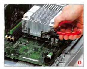
With the heat sink out of the way, the processor card is now exposed. Use a magnetized Phillips screwdriver (you don't want those small screws to fall into the computer) to undo the screws that hold the processor card in place.
