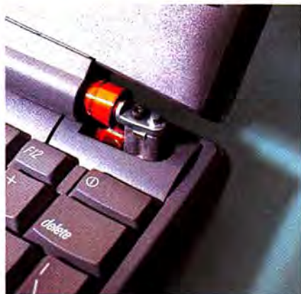
Figure 1 • They're small but dangerous. These screws in the PowerBook 500-series Macs can loosen over time, which can result in a cracked PowerBook case.
