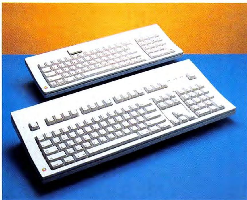
Keyboards come in two flavors: big (81-key) and bigger (105-key). You get to pick which one you want. Both have the on/off switch for the whole system on them. The bigger unit has a row of configurable function keys, just like other computers.
