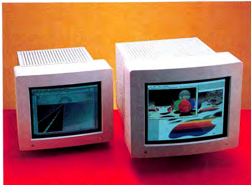
When you get your Mac II, you'll have a choice of monitors. The 13-inch color monitor and the 12-inch black and white monitor both have 480 x 640 x 16 pixel resolution. Yep, each pixel can have one of 16 shades. The richness of the images have to be seen to be believed. The color monitor requires an internal color board.
