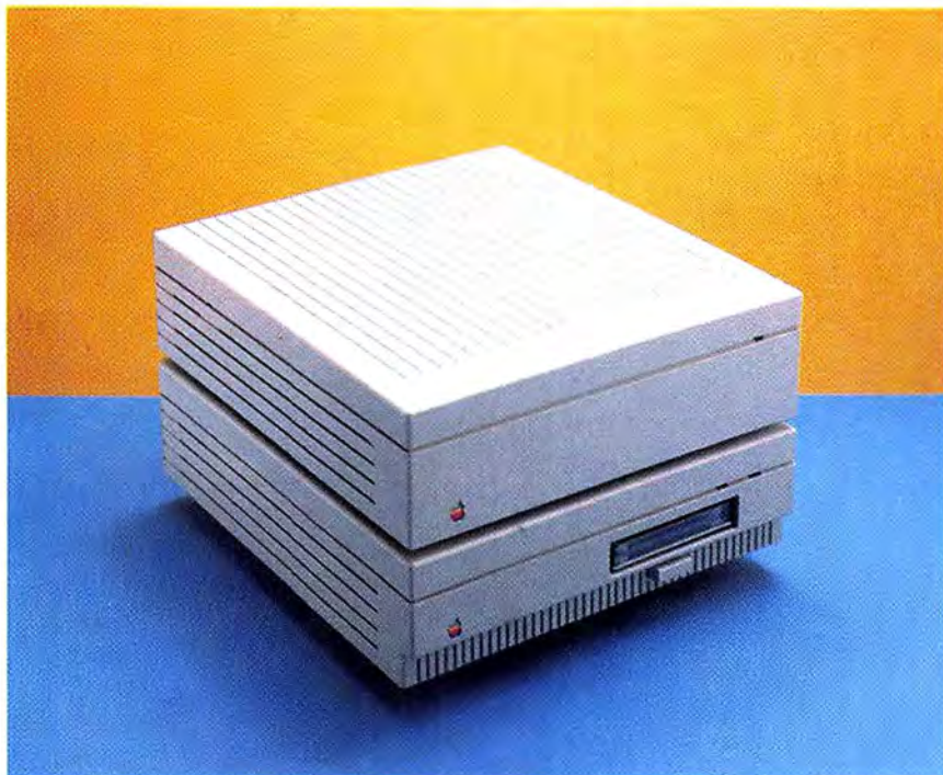
No, it's not the Personal LaserWriter. These two external hard disks will work with any Mac with a SCSI port. The 40-meg unit on the bottom has a built-in tape backup system.
