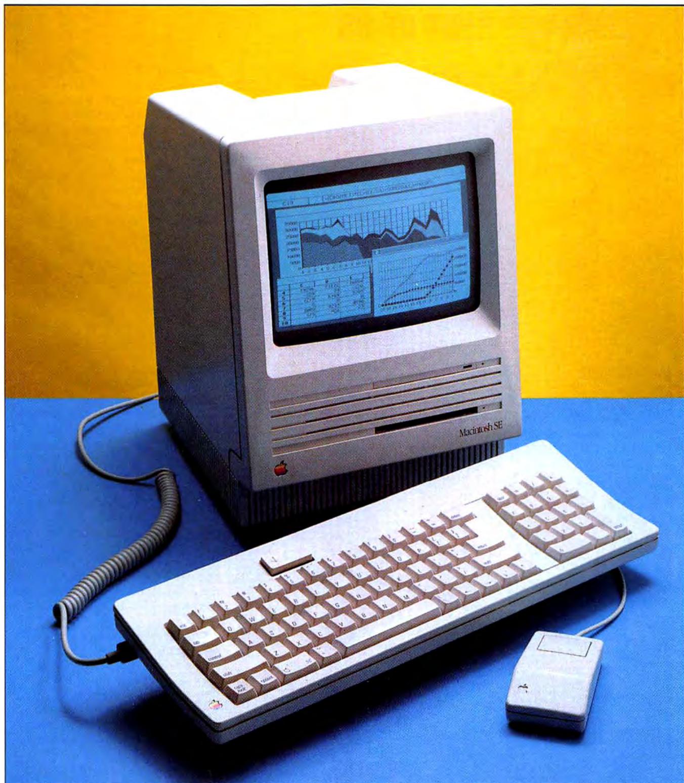
The Mac SE is a very enhanced Mac Plus. What you can't see is the beefed up power supply and the internal fan. This machine is built to have an internal hard disk.
