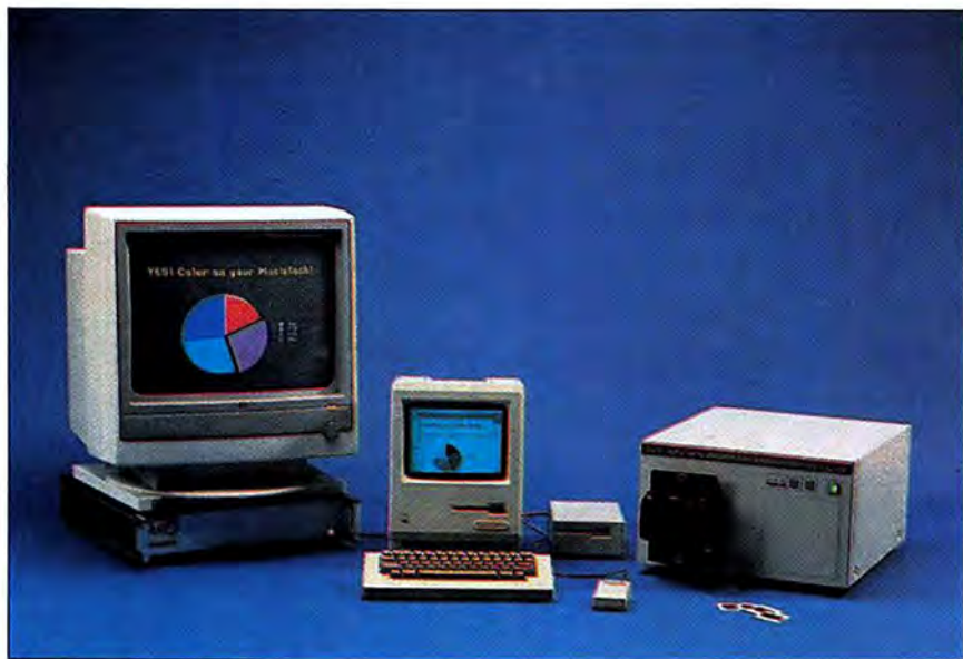
The Dunn Color Macintosh System includes a graphics controller, 19-inch color monitor, film recorder and software.
