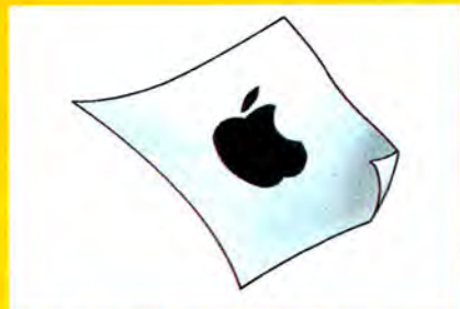
Fig. 5: ...where it attracts the positively charged toner and forms an image on the page
