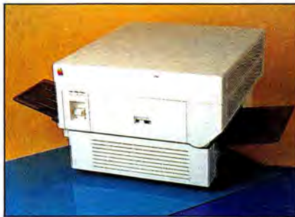
Apple's LaserWriter is the most powerful computer Apple sells. It hooks to the Mac via AppleTalk and is required if you want to print top quality graphics.
