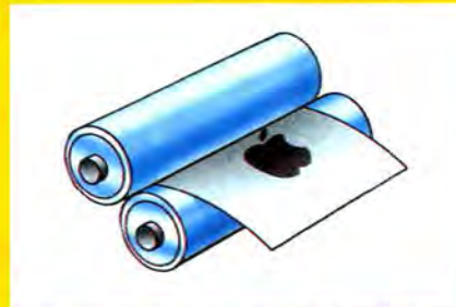
Fig. 6: Finally, the paper holding the toner is passed between heated rollers which "fix" the toner on the page
