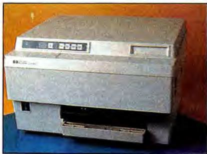
Hewlett-Packard's LaserJet comes with only one font, but accepts others (in cartridges that go in the slot at the top right). It is easy to hook up to the Mac.
