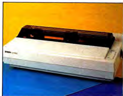
Epson's LQ-1500 is a high-speed, near letter quality (NLQ) printer. It can produce output virtually indistinguishable from a daisywheel printer.
