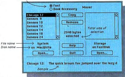
Fig. 6: The Font/DA Mover lets you install and remove fonts and desk accessories.
