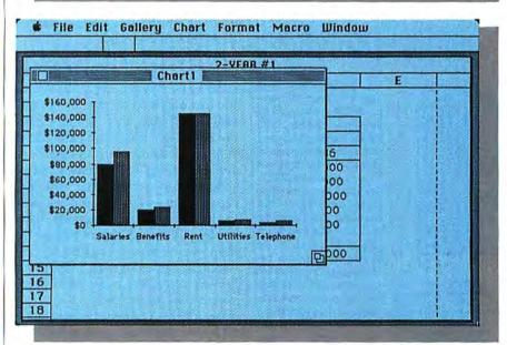
Fig. 2: Charting your spreadsheeted data is easy with *Excel*. First the information to be charted is selected by dragging the mouse on the spreadsheet, which highlights the data. Then "New" is chosen from the "File" menu (top). "Chart" is picked from a dialog box and a new chart is quickly windowed (bottom).
