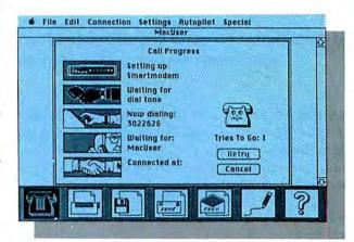
Fig. 3: Smartcom II highlights each step in its call animation, letting users know the current state of the connection. The telephone's eyes move farther down as each step is completed.
