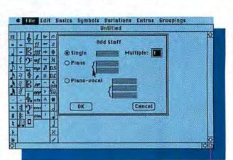
Fig. 3: When creating a new file, the user can select the format of the staves to be used; up to 40 staves may be specified for multiple parts. Also note the columns of symbols on the right hand of the screen: these are the principle tools in *Professional Composer*.
