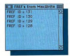
Fig.4: FREF or file reference resources. FREFs tell the Finder which icon goes with which resource. FREF ID = 128 is associated with the application icon. FREFs 129 and 130 are associated with the document icons. FREF 131 is not used by the finder.
