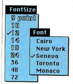
Fig. 1: The fonts and sizes available from most applications show on menus; the outlined numbers are the sizes actually installed in the system. Although you can select the solid numbers, the characters in those sizes will not be perfectly formed.
