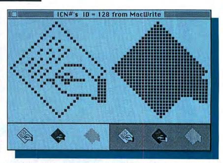
Fig. 1: The icon-list editor window of ResEdit prototype #0.7. This is the standard *MacWrite* icon. The top part of the window is the working area, which is like the FatBits option of *MacPaint*. The bottom sections show the icon, its mask and its "not available" image against both white and patterned backgrounds.
