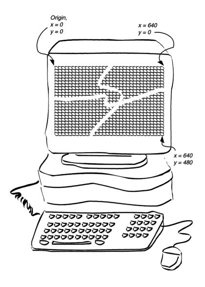
Figure 3-1. The pixel layout in a frame store
