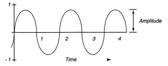
Figure 11-1. Sound as waveform
