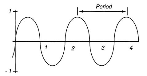
Figure 11-3. Measuring frequency
