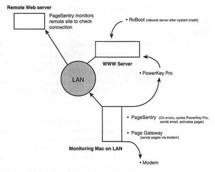
Figure 13.9 The ultimate site monitoring system.
