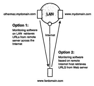
Figure 13.1 Two methods of checking Internet connections.
