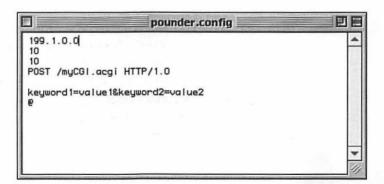
Figure 12.10 A Pounder configuration for a POST method request.
