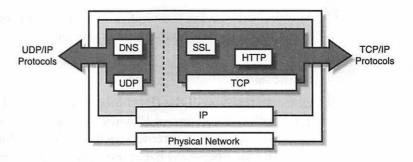
Figure 3.1 The layering of protocols on the Internet.
