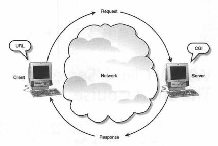
Figure 2.1 Elements of a typical Web client/server transaction.
