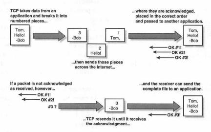
Figure 3.3 How TCP handles missing packets.
