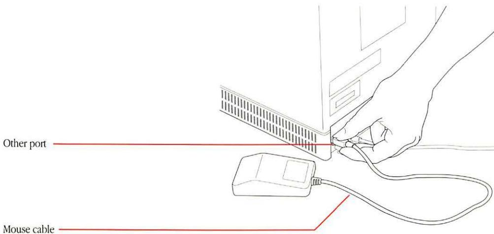
You might prefer to **daisy-chain** the mouse to the keyboard, using the second port on the keyboard rather than the port on the back panel of the computer. It's up to you. Here are some possibilities:
