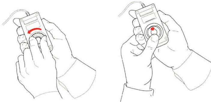
**2. If you have the mouse on the left, hold one hand over the ball and ring to catch them, and turn the mouse back right side up. If you have the mouse on the right, lift the ring off the mouse, hold one hand over the ball, and turn the mouse back right side up.**
