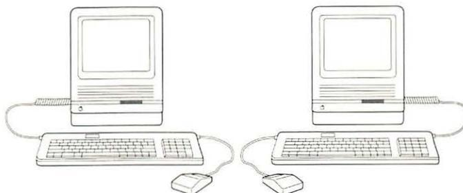
If you have other Apple Desktop Bus devices to attach to your system—a graphics tablet, a joystick, or another keyboard, for example—you can either daisy-chain them to the keyboard or use one of the Apple Desktop Bus ports on the computer's back panel.
