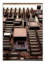
With 386 power and true AT software compatibility, your business, desktop publishing and engineering applications will get a boost to boast about! **Technical Features** • 16 MHz 80386 • 1 Megabyte of 100 nsec 4-way interleaved RAM • PC/AT compatible I/O and BIOS for support of OS/2 • Seven 8-bit expansion slots • Two 16-bit expansion slots • One 32-bit RAM expansion slot • Optional 16 MHz 80387 math coprocessor (\$695)
