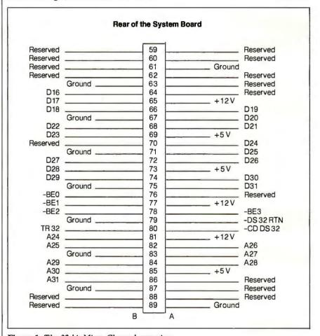
Figure 1: The 32-bit Micro Channel extension.
