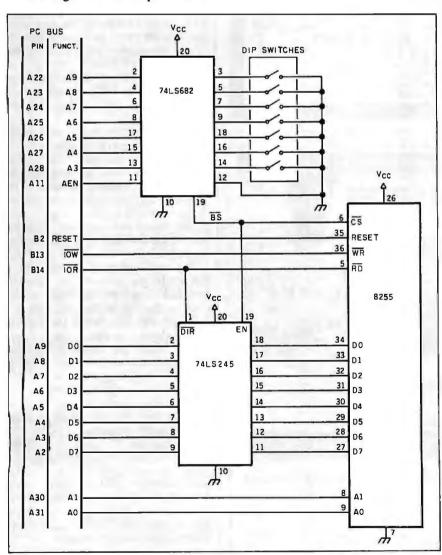
Figure 4: A minimal interface circuit using the 8255. The 8255 response time is sufficient, so you don't need to use I/O CH RDY to extend PC I/O cycles. You do not use address line A2.
