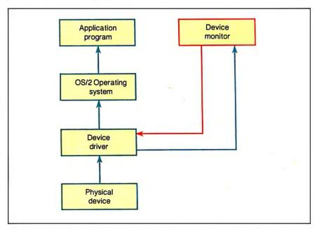
Figure 1: The left side of this diagram shows the normal flow of data from a character device to an application. Registering a device monitor changes the flow to add the box on the right. The characters are passed from the driver to the device monitor in packets, where they can be translated or deleted, and new characters can be added. The characters are then passed back to the driver and from there flow through the operating system to the applications.
