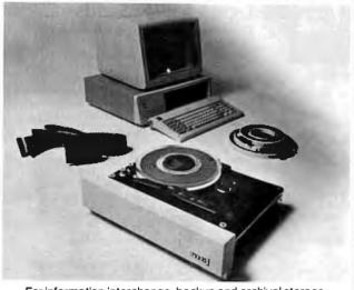
For information interchange, backup and archival storage, AK Systems offers a 9-track, IBM format-compatible ½" magnetic tape subsystem for the IBM PC, featuring:
