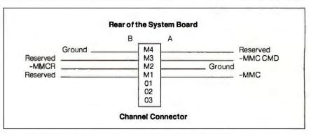
Figure 2: The matched-memory extension to the 32-bit Micro Channel.
