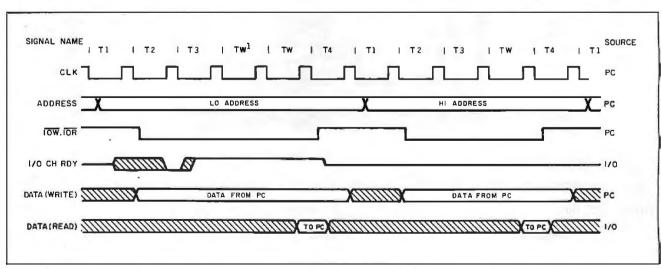
Figure 2: Timing signals for an IBM PC word I/O cycle. The CLK interval is 210 ns. Note that the word cycle is actually two byte I/O cycles and that I/O CH RDY is used to add an extra clock cycle to the first I/O cycle.
