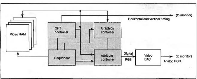
Figure 3: The VGA subsystem. Components of the VGA chip are outlined in red.
