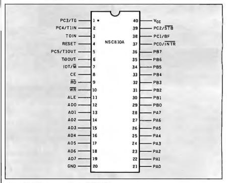
Figure 11: The pin-outs for the NSC810A.
