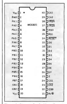
Figure 8: Pin-outs for the Motorola MC6821.
