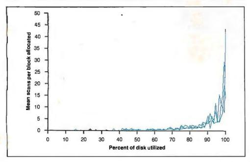
Figure 3: The same as figure 2, but the next-fit algorithm was used, and mean file sizes for three runs are 0.5, I, and 2 percent of disk capacity. Note that the number of scans remains at a constant low level until the utilization reaches 90 percent.
