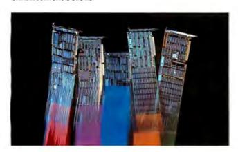
**386 Express**<sup>™</sup> — Our 16-MHz 80386 accelerator — specially suitable for LANs — will make your IBM AT two to three times more productive *and* maintain full software compatibility including OS/2, all at a remarkably low price — \$995.
