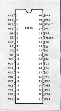
Figure 3: Pin-outs for the Intel 8255.
