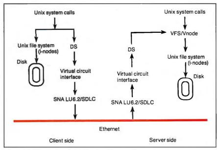
Figure 2: The structure of the Distributed Services file system.
