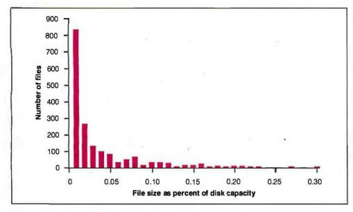
Figure 1: Typical file-size distribution over a hard disk, expressed in percent of hard disk capacity.
