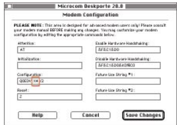
figure 1 / To make your modem do blind dialing (dialing without waiting for a dial tone) when you're using America Online, navigate to this window from the Finder and change X4 in the Configuration field to X1.
