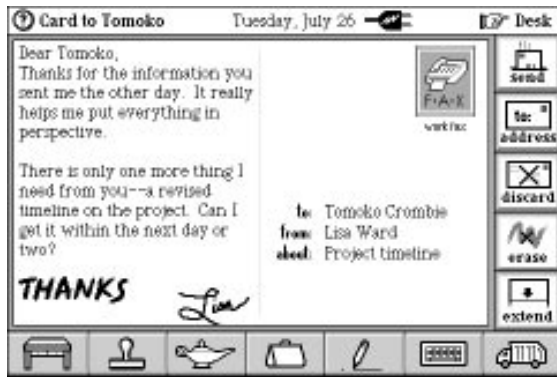
figure 1 / True automation of communications is the strength of General Magic's Magic Cap operating system. It lets you send faxes, e-mail, and pager messages from within many applications. The icon bar at the bottom is for accessing tools and navigating Magic Cap.
