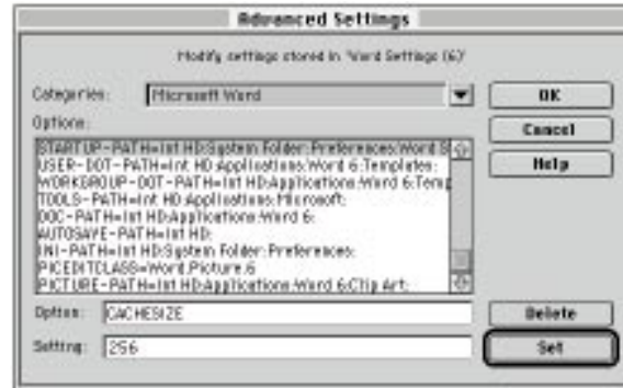
figure 1 / Word 6's hidden Advanced Settings dialog box lets you allocate extra memory to open documents, but how to specify settings isn't obvious. Here, I typed the CACHESIZE option name and setting over those for STARTUP-PATH.
