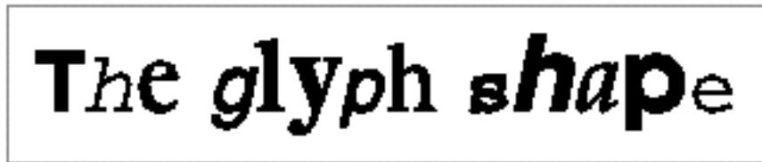
Figure 4-8 An example of a glyph shape with a style run for each glyph
