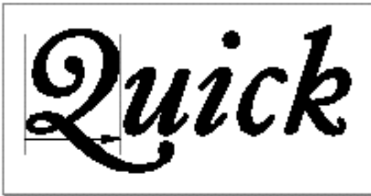
Figure 8-5 Apparent kerning caused by a glyph that extends beyond its advance width
