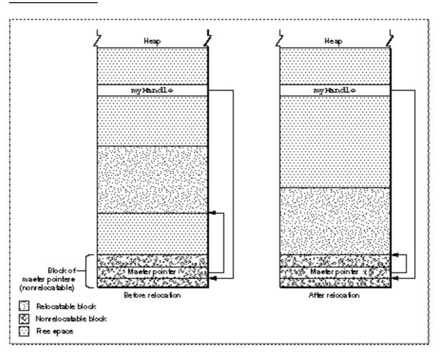
Figure 1-9 A handle to a relocatable block
