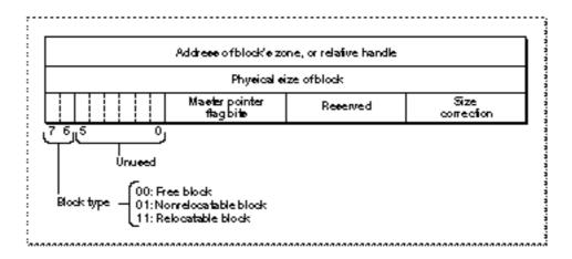
Figure 2-2 A block header in a 32-bit zone
