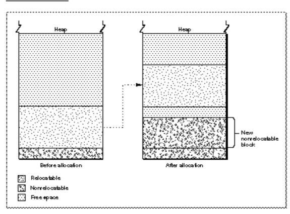
Figure 1-11Allocating a nonrelocatable block
