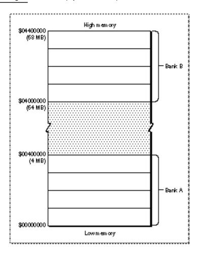
Figure 3-3 The physical address space on a Macintosh IIci with 8 MB of RAM
